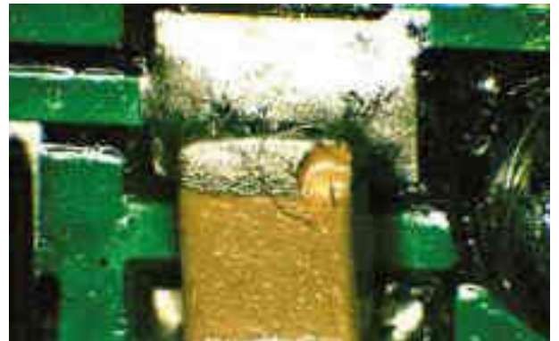
Bad solder joint
