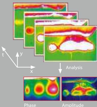
The software IRBIS® 3 active offers comfortable access to the entire active thermography data, starting with the selection and setting of the excitation parameters through to the analysis data.
