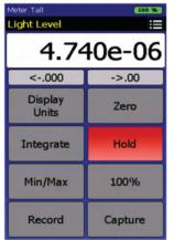
**Meter Screen** provides a large numerical display which allows customers to easily view the measurement data. While using Meter, customers can also perform many processes including:
