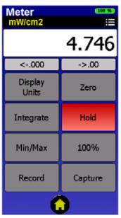
Flash is designed for measurement of pulsed light sources such as Xenon Pulse UV lamps. It includes a flash count, profile of the peak of the flash, as well as
