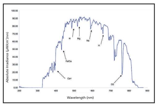
Absorption bands of atmospheric elements are easily identifiable in this solar irradiance spectrum measured with a USB2000+ spectrometer and cosine corrector.
