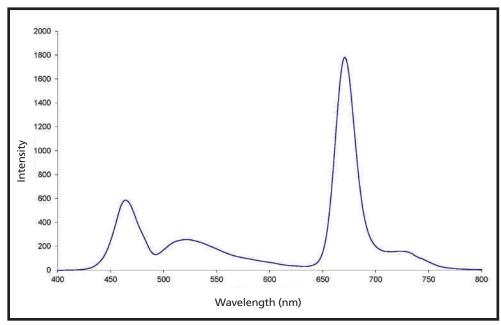
Chlorophyll in water is measured with a USB4000 configured for fluorescence. A 450 nm LED was used for excitation and a cuvette holder for the sample.
